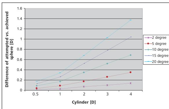
Fig. 8: Calculated spherical error for a toric intraocular lens displaced by a certain angle as a function of the power of the preoperative astigmatism.
