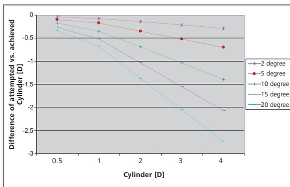
Fig. 9: Calculated cylinder error for a toric intraocular lens displaced by a certain angle as a function of the power of the preoperative astigmatism.
